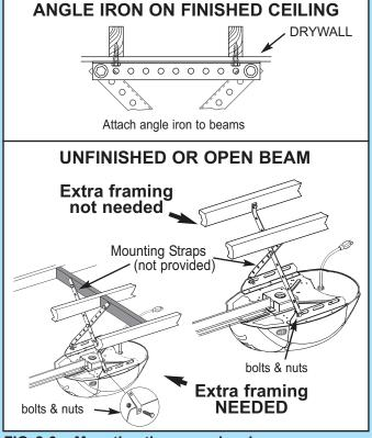
FIG. 2-6 Mounting the power head.
